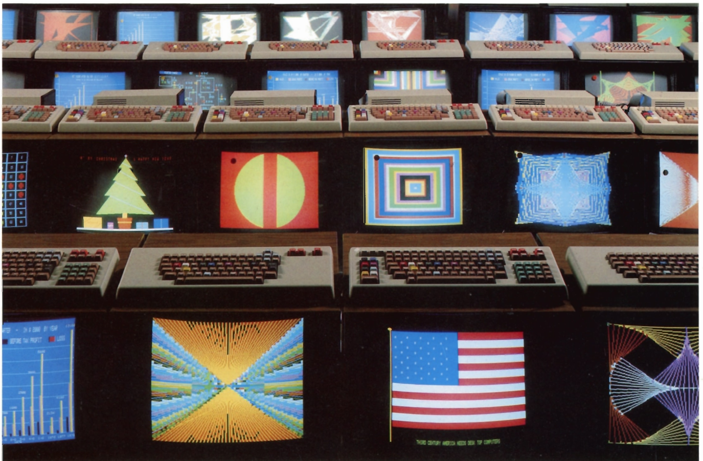
The burn-in line: When ISC units are completed, they run continuously for seven consecutive days, 24 hours a day, before being shipped out of the plant. This extensive burning-in process is an important step that ISC takes to insure customer satisfaction and faultless machine operation.
